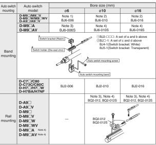
Note 1) Set part number which includes the auto switch mounting band (BJ2-006) and the holder kit (BJ5-2/Switch bracket: Transparent).
