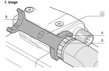
• Apply tool 1 with the correct fork opening (A)/(B) to the screw-type lock (D).
