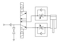
\* A certain amount of leakage is allowed in the specifications of this product. Please note that it is not suitable for holding over an extended period of time.
