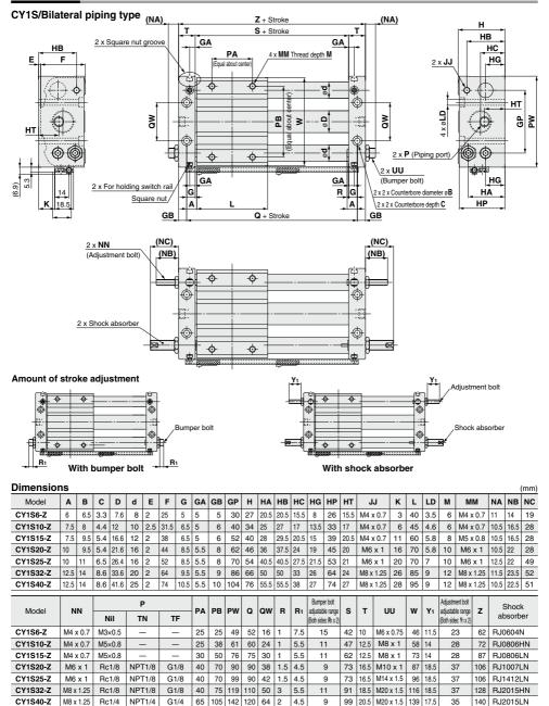
Note) The above figures show the product with auto switches. Auto switch and switch spacer are shipped together with the product, but not assembled.
