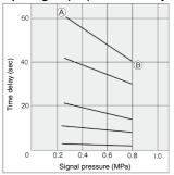
Example) (A) is the point, which is set by the input signal pressure 0.25 MPa, with a delay time of 60 sec. With the same status, if the input signal pressure is increased to 0.8 MPa, the delay time varies to the ® point
