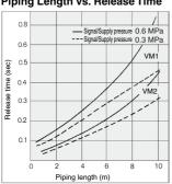
If the input signal (PIL) is turned OFF, the release time of the time delay valve changes depending upon the effective area of the valve and the length of piping. Please refer to the above graph for the standard values.
