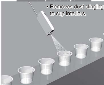
Neutralizing static electricity from plastic cups
