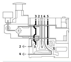
This pressure regulator regulates the pressure in duct 2 after the pressure medium flows through the valve. During exhausting, the air flow in the valve is exhausted from duct 2 to duct 3 via the pressure regulator.
