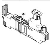
An adjustable pressure regulator can be installed between the sub-base and the valve in order to control the force of the triggered actuator.
