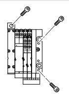
The MPA valve terminal is screwed onto the mounting surface using six M4 or M6 screws. The mounting holes are on the left end plate (CPX) and on the right end plate MPA.
