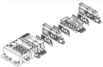
The modular design of the MPA enables outstanding flexibility right from the planning stage and offers maximum ease of service in operation. The system consists of sub-bases and valves.
