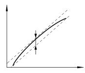
A perfectly linear progression of the control characteristic of the output pressure is theoretical. The maximum percentage deviation from this theoretical control characteristic is referred to as the linearity error. The percentage value refers to the maximum output pressure (full scale).
