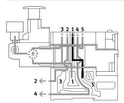
The reversible A regulator splits the working air in duct 1 and regulates the pressure upstream of the valve in duct 5 (the unregulated pressure from duct 1 is in duct 3). The regulated air is then routed to duct 4. The valve is thus operated in reverse mode.
