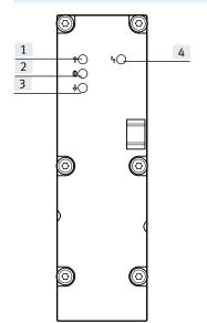
The pressure sensor uses three LEDs to indicate whether the applied pressure exceeds, conforms to or hasn't reached the setpoint value. An additional LED indicates common errors (limit exceeded or not reached).
