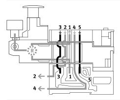
This pressure regulator regulates the pressure upstream of the valve in duct 1. Ducts 2 and 4 thus have the same regulated pressure. During exhausting, the exhaust flow in the valve is from duct 2 to duct 3 and from duct 4 to duct 5.
