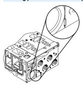
MPA offers a number of options for creating pressure zones if different working pressures are required. Depending on the electrical interface, up to 16 pressure zones are possible.
