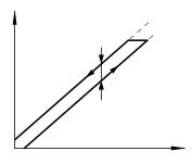
There is always a linear relationship within a certain tolerance between the setpoint value entered and the pressure output. Nevertheless, it makes a difference whether the setpoint value is entered as rising or falling. The difference between the maximum deviations is referred to as hysteresis.
