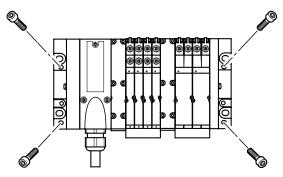
The MPA valve terminal is screwed onto the mounting surface using four M4 or M6 screws. The mount-
