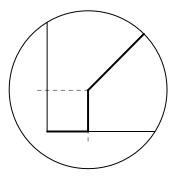
In practice, there can be a residual voltage or residual current at the setpoint input of the VPPM via the setpoint generator.
