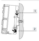
The valve terminal MPA is hooked onto the H-rail → arrow [1].
