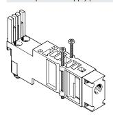
This vertical pressure supply plate enables an individual valve to be supplied with individual operating pressure independently of the operating pressure of the valve terminal.
