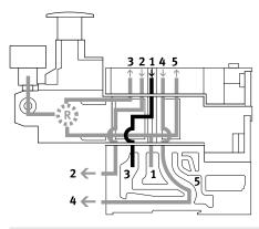
The reversible B regulator splits the supply air in duct 1 and regulates the pressure upstream of the valve in duct 3 (the unregulated pressure from duct 1 is in duct 5). The regulated air is then routed to duct 2. The valve is thus operated in reverse mode.
