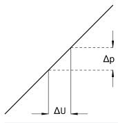
The response sensitivity of the device determines how sensitively one can change, i.e. adjust, a pressure.
