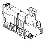
Additional functional units can be added to each valve position between the sub-base and the valve.
