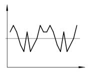
The repetition accuracy is the margin within which the fluidic output variable is scattered when the same electrical input signal coming from the same direction is repeatedly adjusted. The repetition accuracy is expressed as a percentage of the maximum fluidic output signal.
