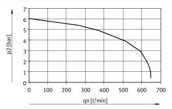
Supply pressure 10 bar, regulated pressure set at 6 bar
