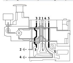
This pressure regulator regulates the pressure in duct 4 after the pressure medium flows through the valve. During exhausting, the air flow in the valve is exhausted from duct 4 to duct 5 via the pressure regulator.
