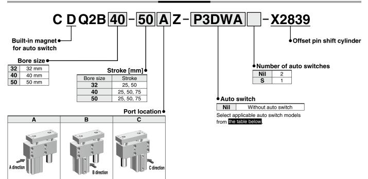
Auto Switch Models: Refer to the Best Pneumatics Catalog for further information on auto switches. Magnetic Field-resistant Auto Switches
