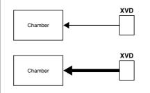
In the initial state, the sub-valve opens and the set amount (needle valve) is supplied slowly into the chamber.
