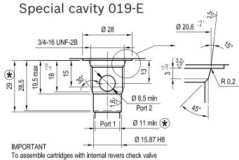
To assemble cartridges with internal revers check valv (VEI-8A-2A-06-VU etc.)
