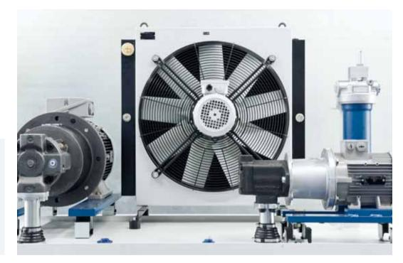
Noise-decoupled motorpump assemblies with optimized suction lines and noise-decoupled, silent oil/air heat exchanger unit of the KOL series
