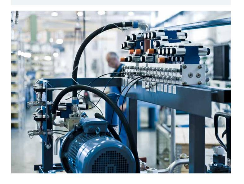
For power unit construction we utilize the world's most comprehensive hydraulics construction kit. Our Rexroth standard components cover all requirements in fine gradations from the compact small power unit to large systems. We combine components from our modular product range to form efficient function groups. Hydraulic manifolds or accumulator stations assembled on this basis can also easily be extended or adapted to new tasks after commissioning.
