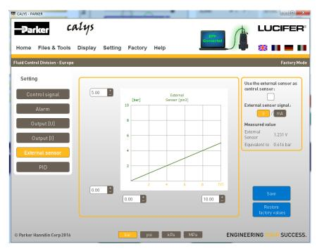
This menu permits the user to configure the settings of the external sensor signal. It is on the Pin 3 of the M12 A connector (see connector details on paragraph 2.4).
