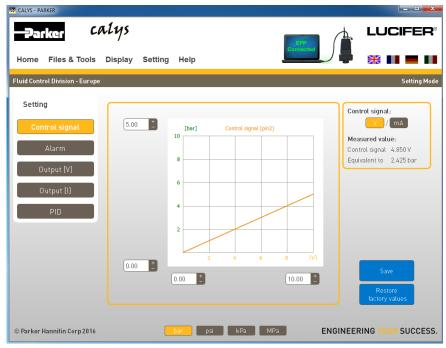
This menu permits the user to change the setting of the regulator reference signal. It is on the Pin 2 of the M12 A connector (see connector details on paragraph 2.4).
