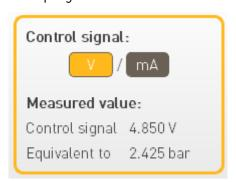
In the same scope, you can read the current analog value of your control signal and see its equivalent value on the output pressure.
